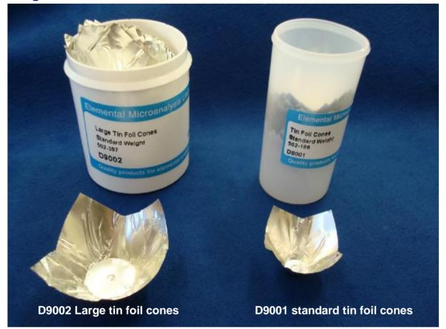
A larger size cone formed from a 50mm suitable for large volume samples. This product is equivalent to Leco  $\circledast\,$  part numbers 502-397 and 502-397-400.
